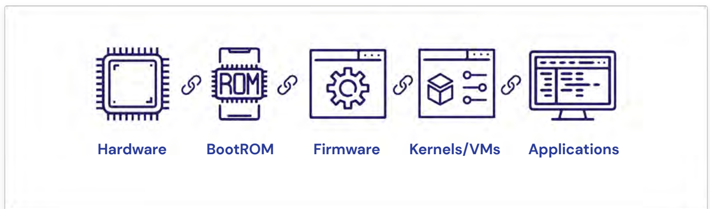
Figure 1: Chain of Trust Connecting System Components from Hardware
